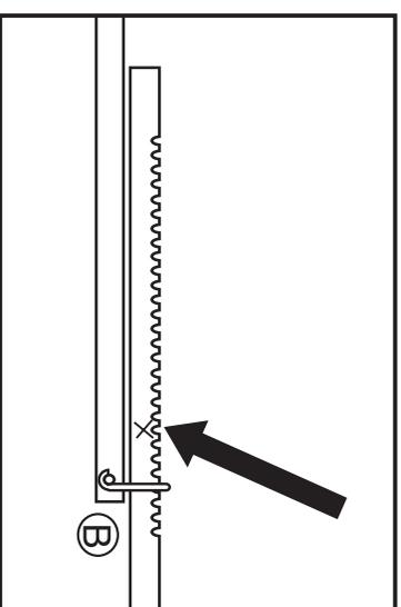
2. Holding loop B straight up, count four notches to left (toward free end) and make a distinctive pencil mark on notched bar. Repeat steps 1 and 2 each time the Hurricane Wedge is to be used at a different location.
