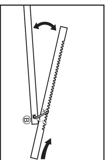
3. Raise notched bar at left (free) end, and position top of loop B into marked notch. Push down on left end of notched bar so Hurricane Wedge expands into position.
